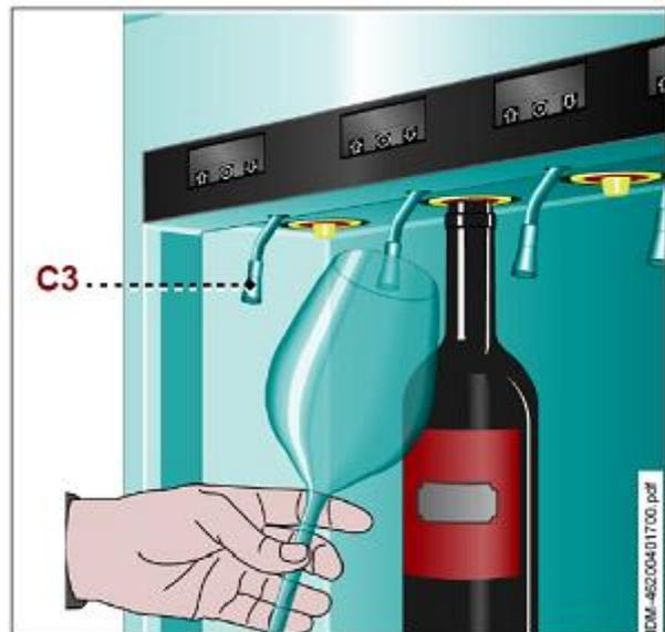
3. Press one of the buttons to supply the desired dose. The wine supply stops when the setting dose is reached.
